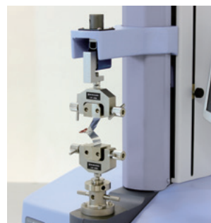
180° Peeling Test on Package Crimping
