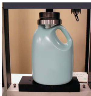
Compression Test of Containers
