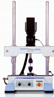
Servopulser EHF Servo-Hydraulic Fatigue and Endurance Tester, Table-Top Type
