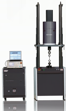
Servopulser EMT Series Electromagnetic Force Fatigue/ Endurance Testing System
