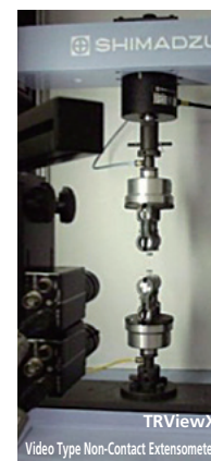
Tensile Testing of Dental Wire
