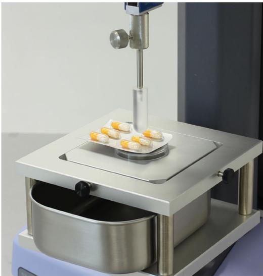
Pill Push-Out Test Using a Pill Push-Out Test Jig Set
