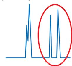
The two separate flows are merged just before reaching the detector, so that data can be acquired as a single chromatogram.
