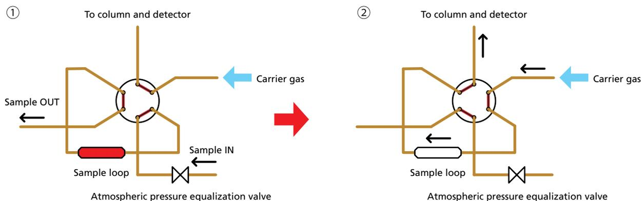
Sample gas flows into the sample loop for a fixed period of time. Then the atmospheric pressure equalization valve is closed to equalize the pressure. Equalizing the atmospheric pressure ensures that a fixed quantity of sample is measured.
