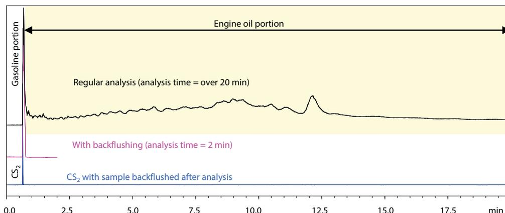
Fig. 3 Chromatogram of Engine Oil Containing Gasoline
