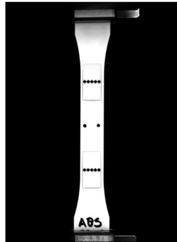
**Figure 1:** Image of sample with flags attached to mark the boundaries of the gage length.
