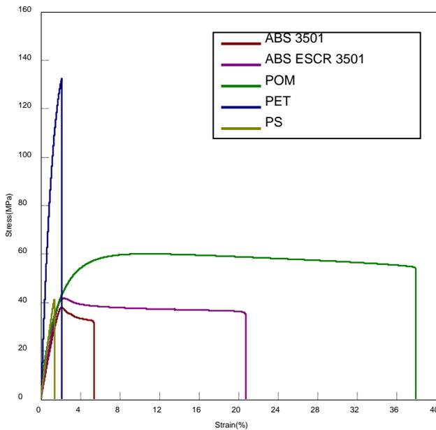
**Figure 2:** Averaged stress strain curves for ABS 3501, ABS ESCR 3501, POM, PET and PS
