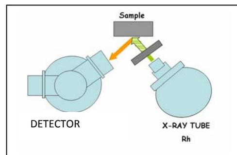
EDX works by a simple process whereby a sample is irradiated by an incidental X-Ray. The sample absorbs the incidental X-Ray and emits characteristic X-Rays for the elements that make up its composition. After analysis the sample is not radioactive or altered in any way.
