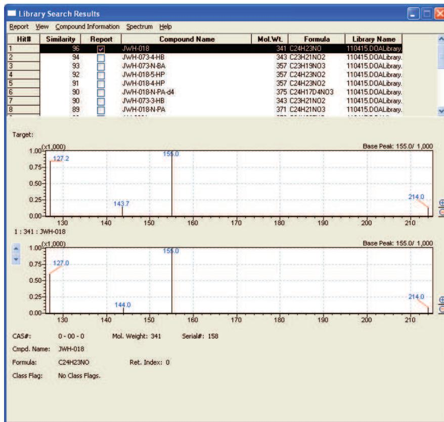
**Figure 6:** Library search results for the tandem mass spectrum of Peak A. The top hit is the designer cannabinoid **JWH-018**. The other hits found are metabolites of synthetic cannabinoids which have different precursor masses and therefore can be distinguished from JWH-018.
