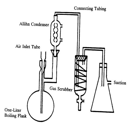
FIGURE 2 CYANIDE DISTILLATION APPARATUS
