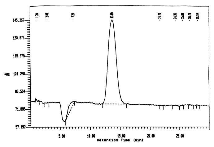
Figure 2. Liquid Chromatogram of glyphosate at 250 ug/L. Conditions are as stated in Table 1.
