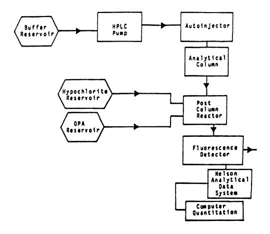
Figure 1. HPLC, Post-Column Reactor System
