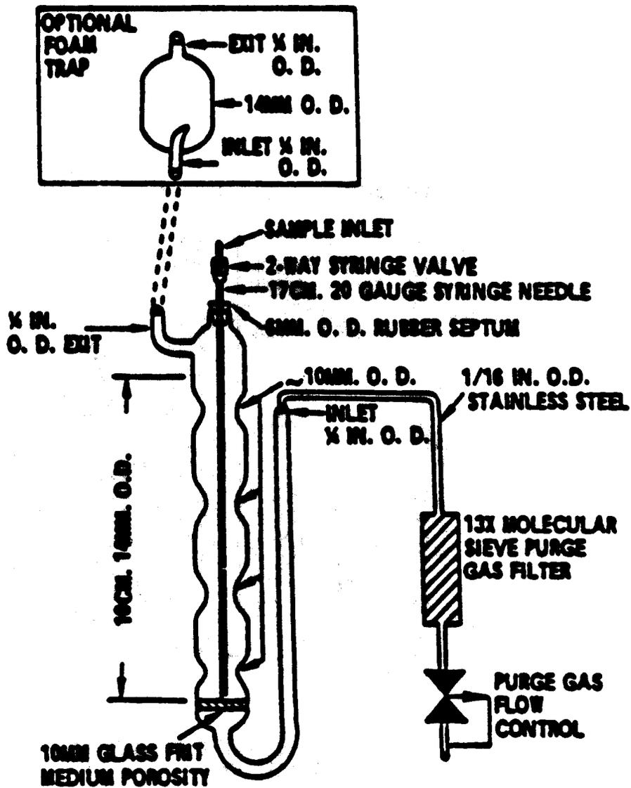
FIGURE 1. PURGING DEVICE
