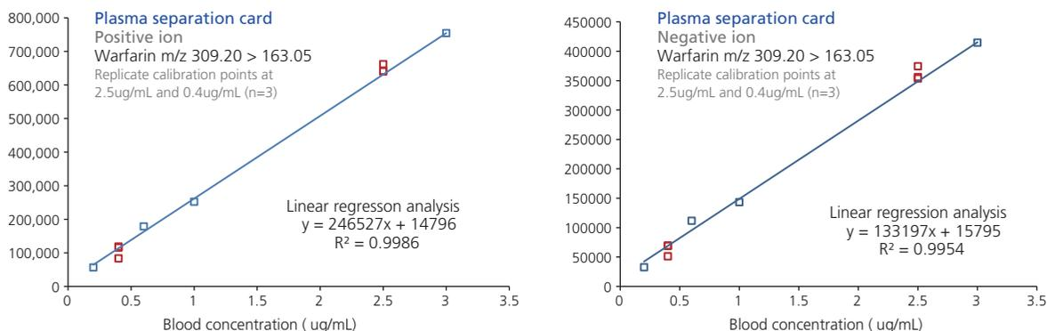
Figure 4. In both ion modes, the calibration curve was linear over the therapeutic range studied for warfarin extracted from PSC's (calibration range 0-3ug/mL, single point calibration standards at each level with the exception of replicate calibration points at 2.5ug/mL and 0.4ug/mL (n=3);  $r^2 > 0.99$  for PSC analysis [ $r^2 > 0.99$  for a conventional plasma extraction]).
