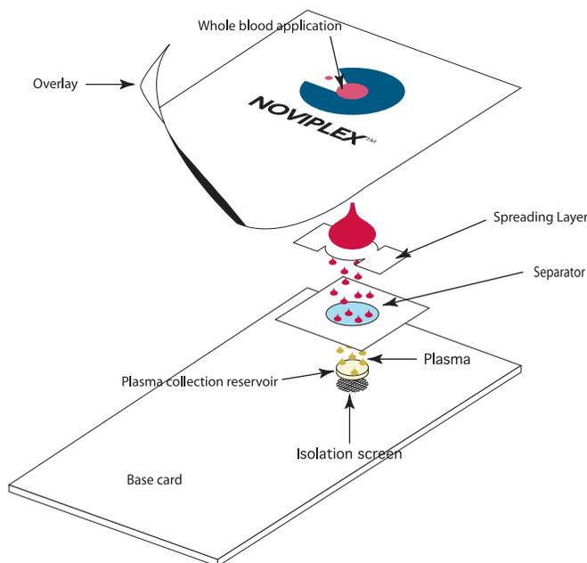
Figure 2. Applying a blood sample, either as a finger prick or by accurately measuring the blood volume, to the laminated membrane stack retains red cells and allows a plasma sample to be collected. The red cells are retained by a combination of adsorption and filtration whilst plasma advances through the membrane stack by capillary action. After approximately three minutes the plasma Collection Disc was saturated with an aliquot of plasma and was ready for LC/MS/MS analysis.
