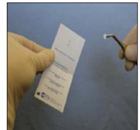
The collection disc is removed from the card and is ready for extraction for LC-MS/MS analysis.
