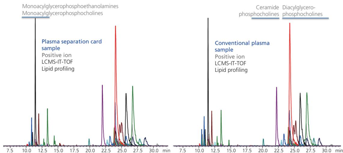
Figure 6. Lipid profiles from the same human blood sample extracted using a plasma separation card (left hand profile) compared to a conventional plasma samples (centrifugation). Both lipid profiles are comparable in terms of distribution and the number of lipids detected (the scaling has been normalized to the most intense lipid signal).
