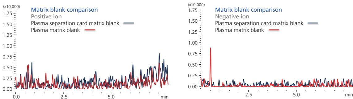
Figure 5. Matrix blank comparison. In both ion modes, the MRM chromatograms for PSC and plasma are comparable. Warfarin ion signals were not detected in the any PSC or plasma matrix blank.
