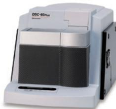
Differential Scanning Calorimeter
