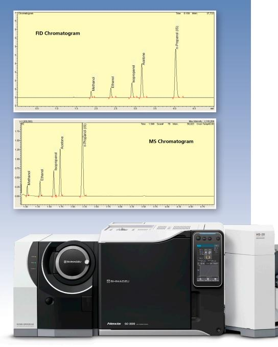
In addition, labs have been adding another step to provide a more confident level of confirmation. They not only compare retention time, but also match the ethanol mass spectrum from the sample to a library spectrum from the known standard.
