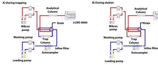
Fig. 2 Flow Diagrams of Trap and Elute System
