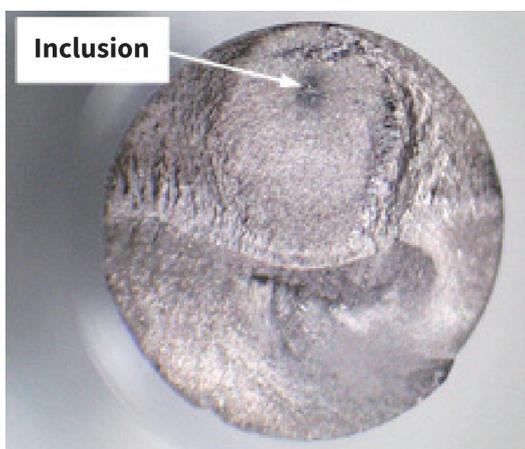
Fig. 7 — Fracture surface of SNCM439 sample.
