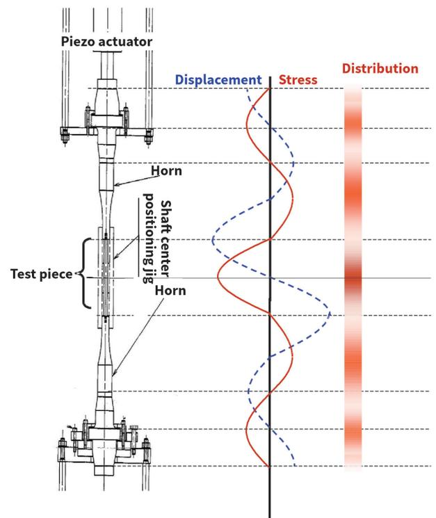
**Fig. 5** — The acoustic wave train can be mounted to a universal test machine with the sample connected to a second horn at the base of the frame to apply a mean stress.
