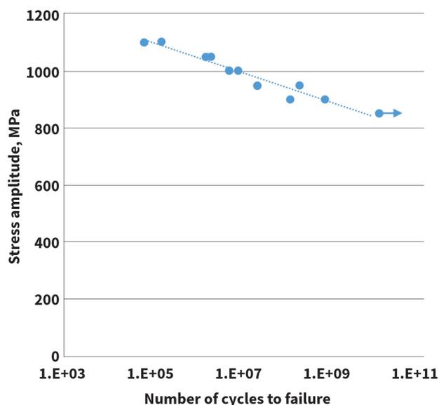
Fig. 6 — S-N curve for SNCM439 steel sample.
