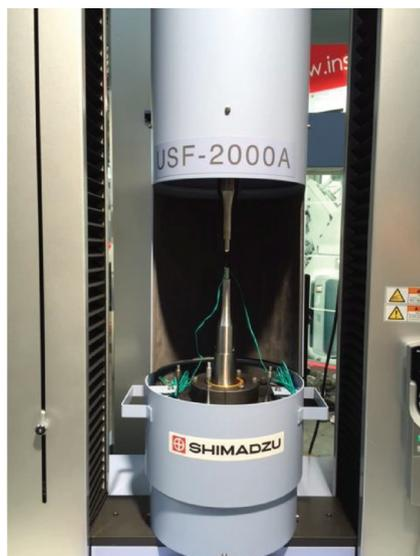
**Fig. 4** — External view of the mean stress loading jig.
