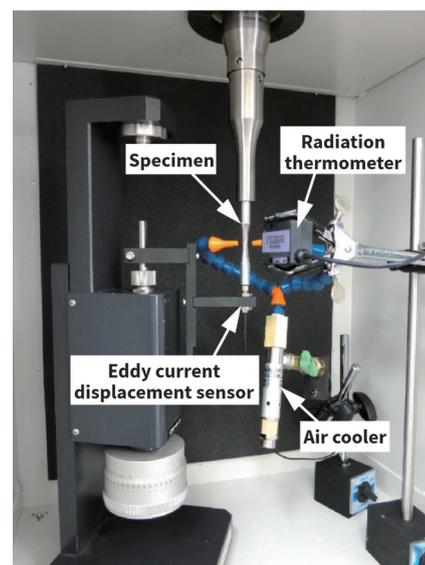
Fig. 2 — Shimadzu USF-2000A ultrasonic fatigue testing system.
