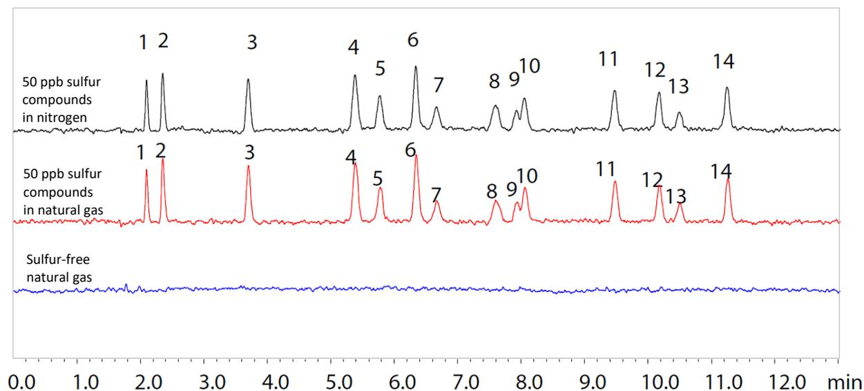
**Figure 4:** Stacked chromatograms showing the SCD-2030 response for a 50 ppb mix of sulfur compounds in nitrogen (black), in natural gas (red), and a blank, sulfur-free natural gas standard (blue). Note that the baselines have been shifted for comparative purposes.
