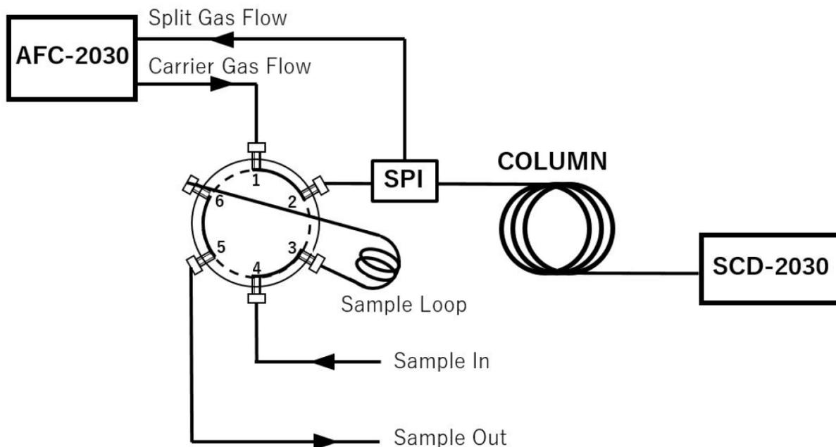
Figure 2: Schematic of instrument configuration.
