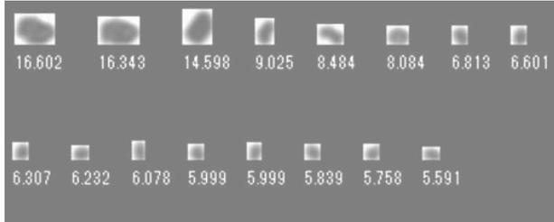
**Figure 9:** Images showing the area equivalent diameter (in  $\mu\text{m}$ ) of the contaminating particles
