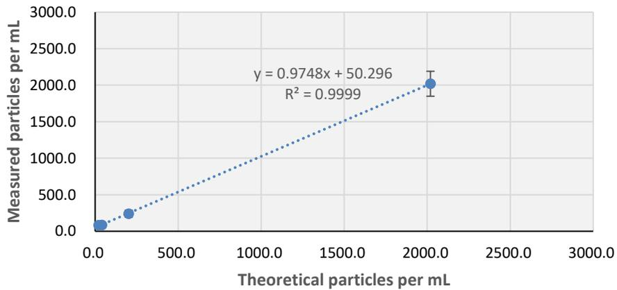
**Figure 4:** Initial scatterplot of 100  $\mu\text{m}$  bead RM data
