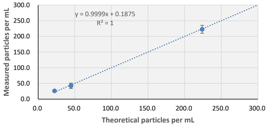
**Figure 13:** Corrected scatterplot of the 20 µm bead RM, showing lower concentrations analyzed in triplicate, a trend line, the regression equation, and the r-squared value
