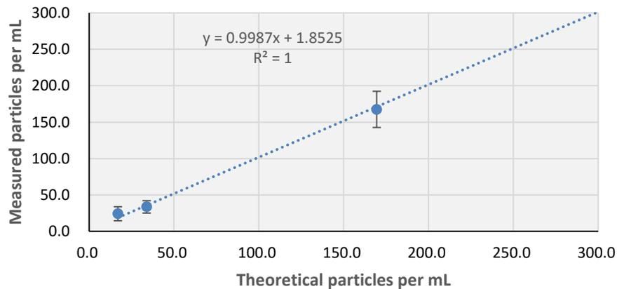
**Figure 11:** Corrected scatterplot of the  $100\ \mu\text{m}$  bead RM, showing lower concentrations analyzed in triplicate, a trend line, the regression equation and the r-squared value
