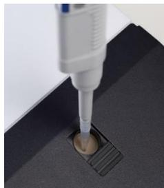
**Figure 3:** Adding Sample to the iSpect DIA-10
