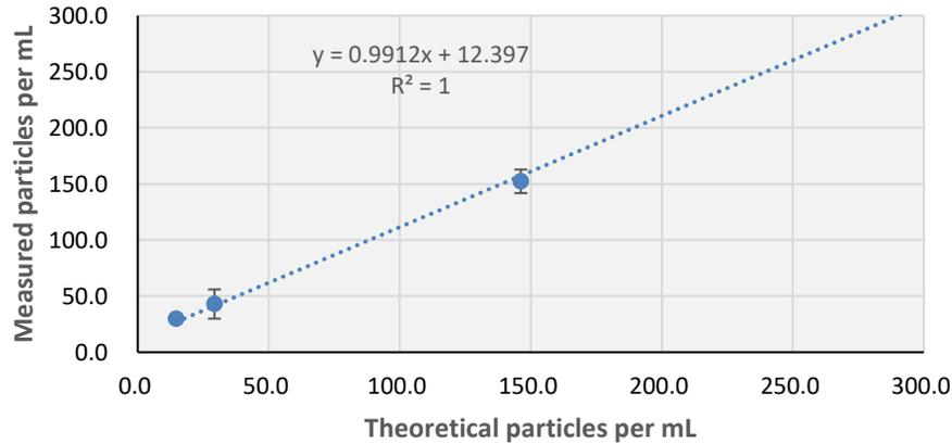
**Figure 14:** Corrected scatterplot of the 50 µm RM, showing lower concentrations analyzed in triplicate, a trend line, the regression equation and the r-squared value
