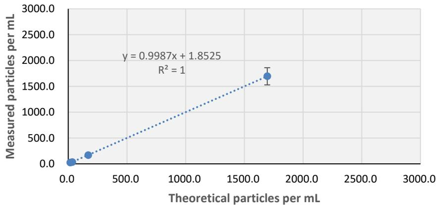
**Figure 10:** Corrected scatterplot of  $100\ \mu\text{m}$  bead RM data showing each concentration analyzed in triplicate, a trend line, the regression equation and the r-squared value
