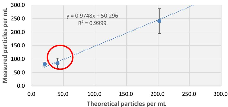
**Figure 5:** Scatterplot of the 100  $\mu\text{m}$  bead RM at lower concentrations only
