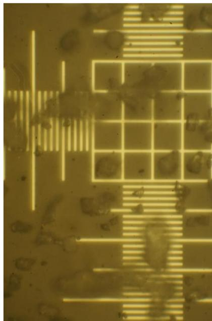
**Figure 1:** IR microscope slide image showing a mixture of particles with calibration lines 10  $\mu\text{m}$  apart (boxes are 50  $\mu\text{m}^2$ )
