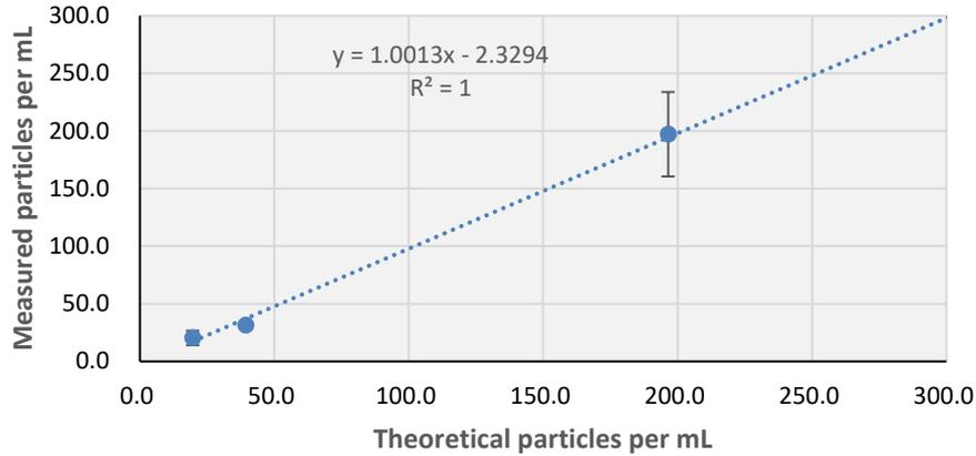
**Figure 12:** Corrected scatterplot of the 10 µm bead RM, showing lower concentrations analyzed in triplicate, a trend line, the regression equation, and the r-squared value
