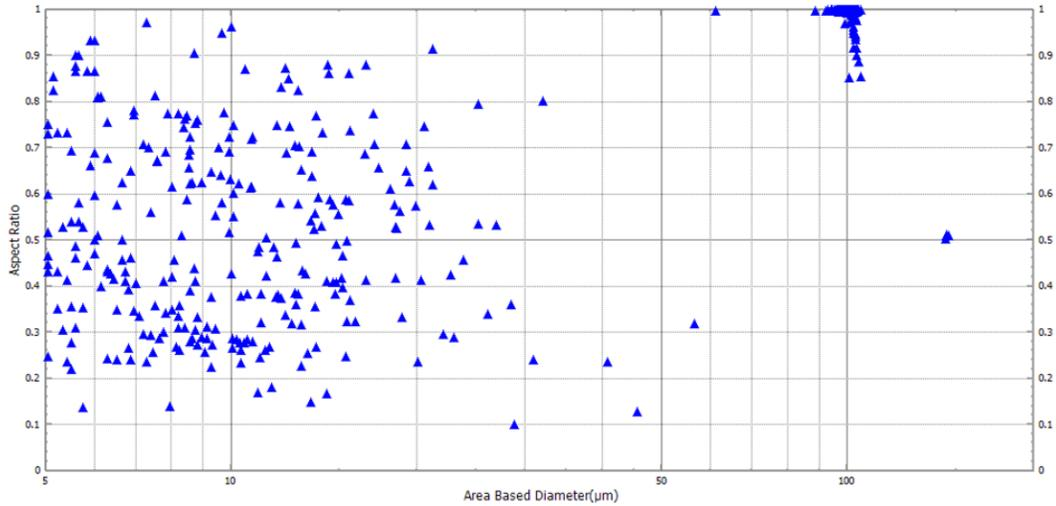
Figure 6: Area-based diameter versus aspect ratio scatterplot of the 100 µm bead RM
