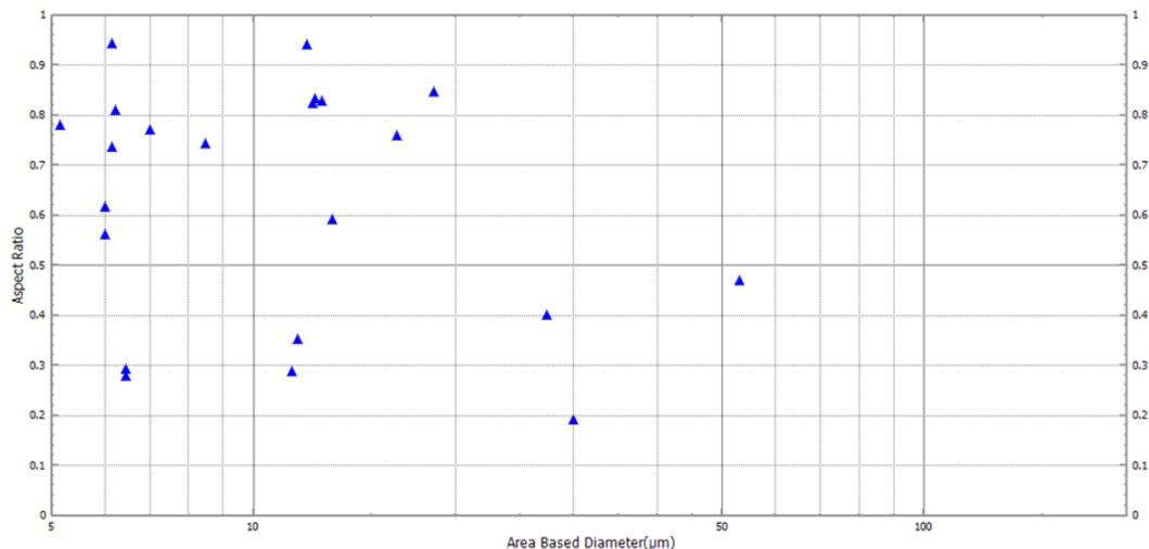
Figure 7: Area-based diameter versus aspect ratio scatterplot of dilution solvent from 15 mL tube prewashed and mixed 20 times
