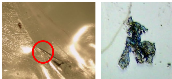
Figure 2: (Left) Visible defect found in plastic packaging viewed with a stereo microscope; (Right) Excised fiber rolled flat on a low-E microscope slide and imaged with the SurveyIR
