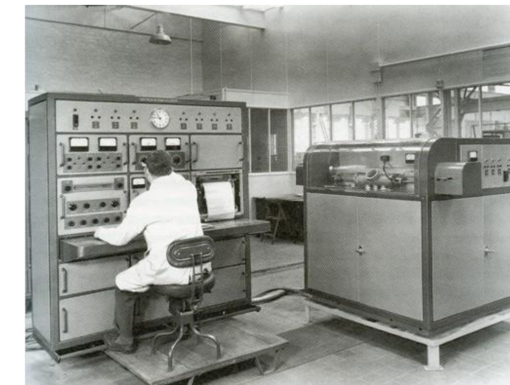
MS5 (1955): Features new thermal ionisation source, a 12 inch radius 90° magnetic sector, with a 6 kV source voltage. Operated by Barry Russell from the test department.
