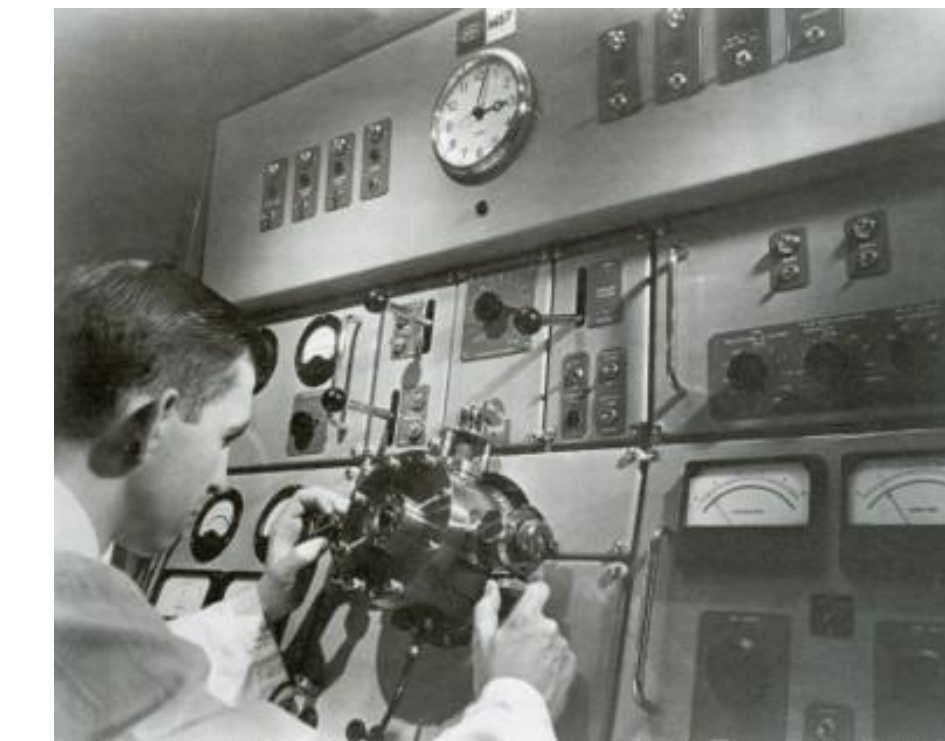
MS7: The spark source Mattauch-Herzog type double focusing sector instrument operated by J. Rogers Woolston at RCA, USA, for analysis of solids in 1961. The first MS7 to reach North American shores, it was actually dropped as a crane removed it from the ship on which it crossed the ocean and sought to deposit it on the dock. In later years, Woolston delighted in telling the story of going up to Newark (NJ) to rescue it.
